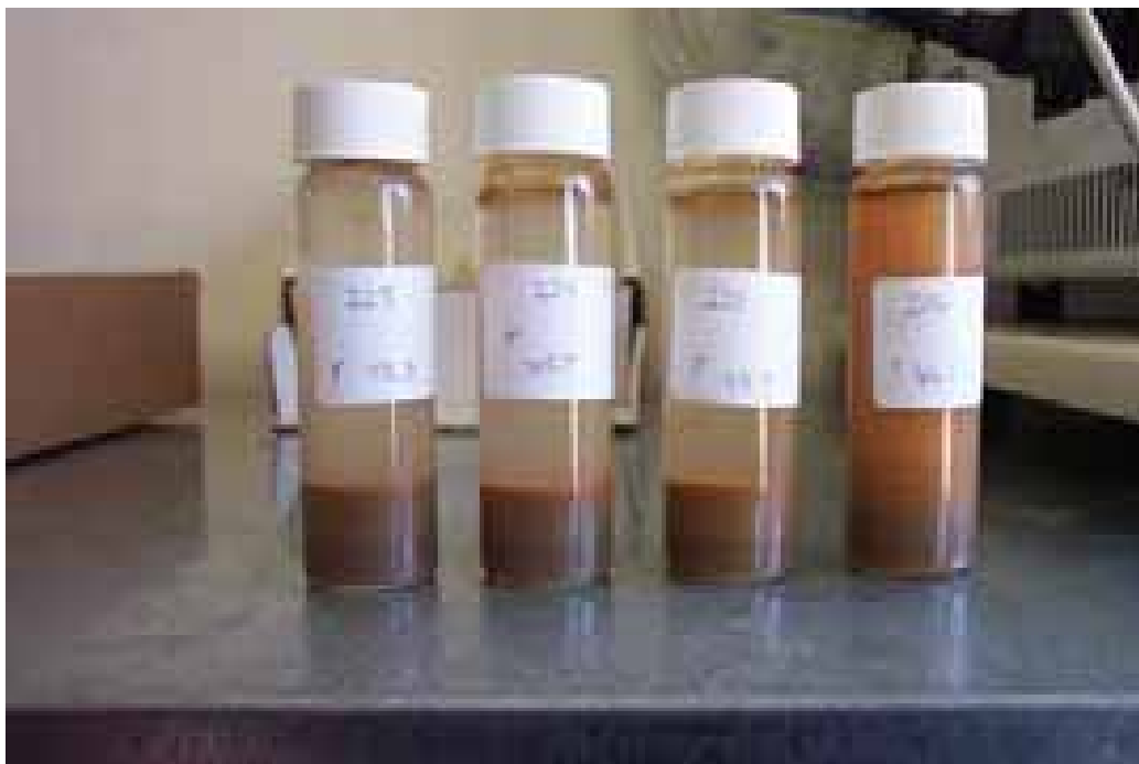
Figure 5-4. Soil samples collected from U12-1807 (30 to 33 feet bgs) containing LNAPL.
